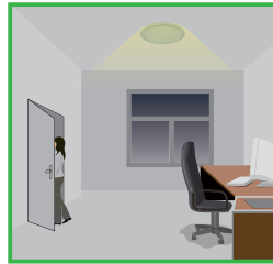
People left, lamp still dims to 0/10%/30%/50% (options) standby level after the hold time.
