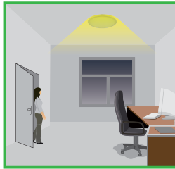
With insufficient natural light, the sensor switches on the lamp automatically when person enters room.
