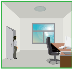
With sufficient natural light, the lamp does not switch on when presence detected.
